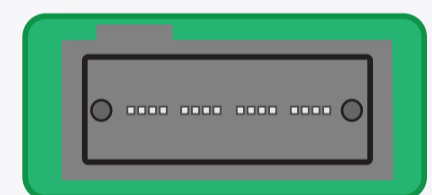
APC MPO Connectors Green Housing (SMF MPO connectors will have either green or yellow) < -65dB Back Reflection
