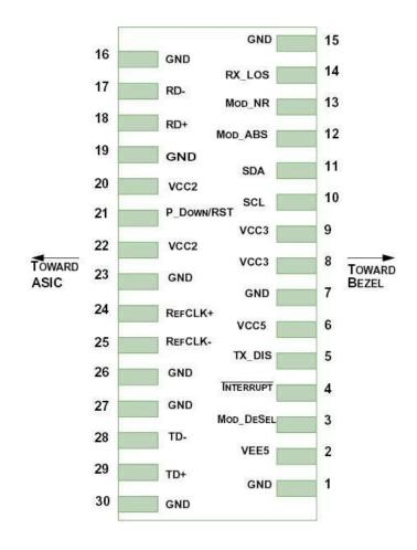
Pin-out of connector Block on Host board
