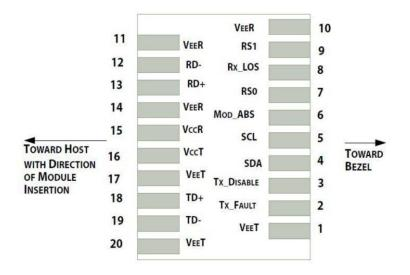
Pin-out of connector Block on Host board
