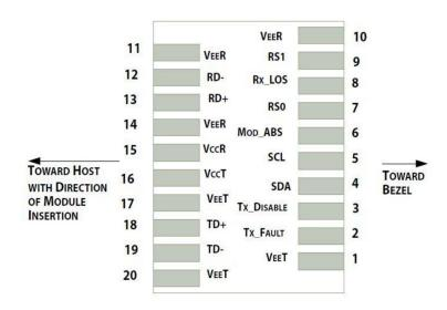
Pin-out of connector Block on Host board
