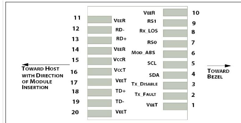
Pin-out of connector Block on Host board
