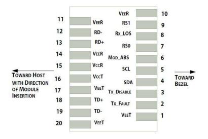
Pin-out of connector Block on Host board
