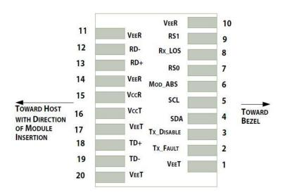
Pin-out of connector Block on Host board
