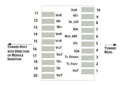
Pin-out of connector Block on Host board
