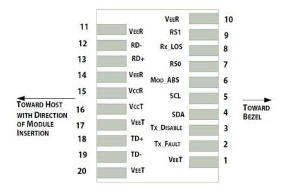
Pin-out of connector Block on Host board
