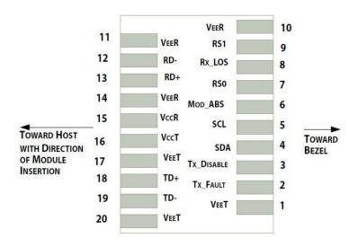
Pin-out of connector Block on Host board
