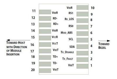
Pin-out of connector Block on Host board
